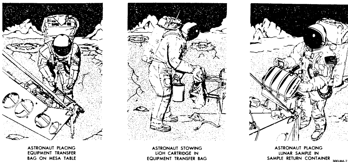
Figure 2.11-16. Modularized Equipment Stowage Assembly Application
